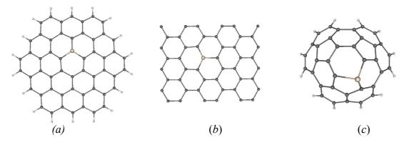
Figure 1: TM-doped circumcoronene (a), TM-doped graphene surface (b), TM-doped C<sub>36</sub> (c).
