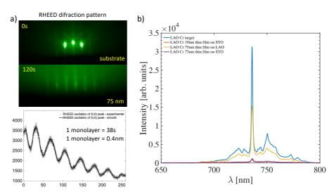
Figure 1. a) RHEED pattern and oscillation obtained during thin film growth. b) Luminescent spectra of different luminescent thin films
